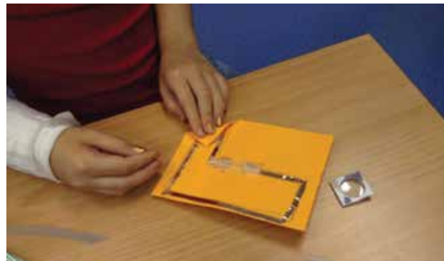
Students use copper tape, LEDs, and coin batteries to build their own circuits to light up greeting cards.
