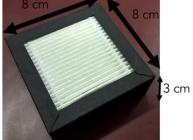
Figure 3. 100% recirculating HEPA filtration system inside the tested desktop 3D printer
