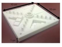
**Figure 1.** Printed standardized test part from NIST used for emissions testing
